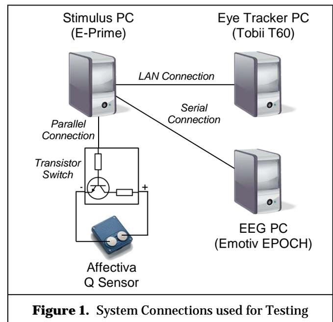
Figure 1. System Connections used for Testing
